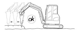
Never run the hydraulic breaker longer then 15 seconds on the same spot. Move the working tool to a new position if the object does not break.
