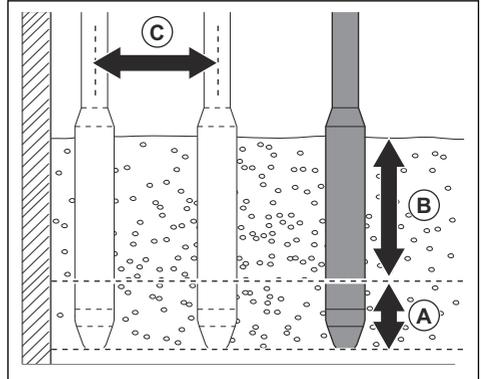
3. Wait approximately 10–20 seconds until the surface around the vibrator head is shiny and no air bubbles come to the surface.
