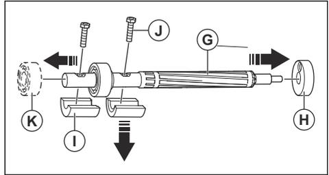
5. Remove the bearing holder (H), the eccentric element (I) and the screws (J).
