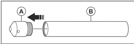
**Note:** The end cap (A) has a right hand thread.
