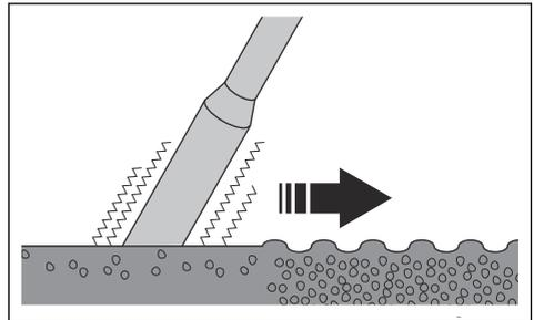
4. Remove the vibrator head slowly to let the concrete fill the hole from the vibrator head.
