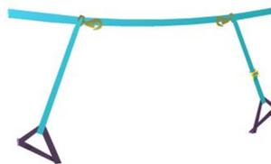
FALLING SAFETY STRAPS FOR SANDWICH PANELS
