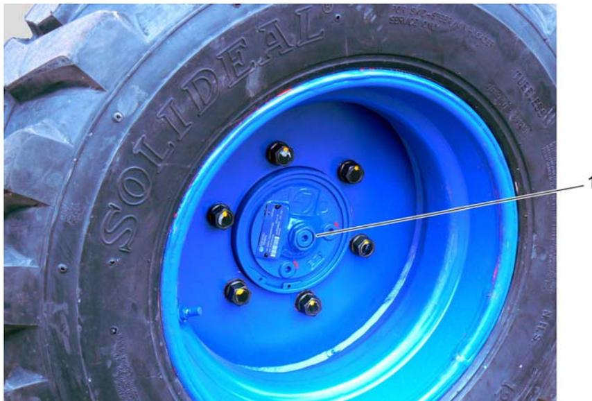
*Bolt for the multiple disc brake*
