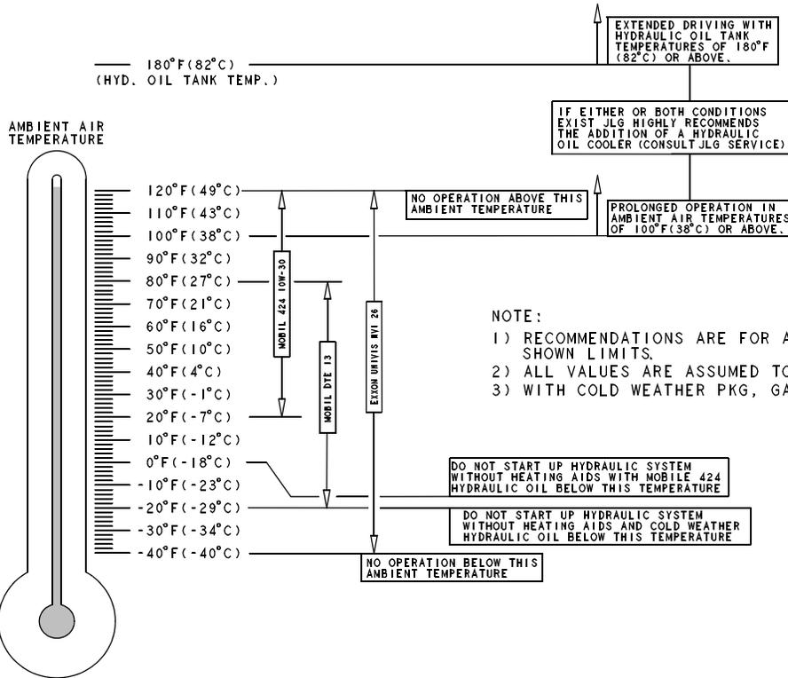
Figure 6-2. Engine Operating Temperature Specifications (Kubota)- Sheet 2 of 2
