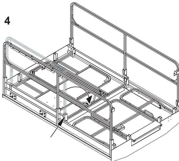
**Figure 4-4. Platform Rails - Fold Down Sequence - Deck Extension Side Rails**
