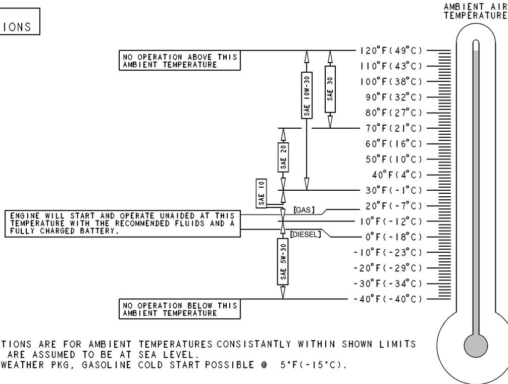
Figure 6-1. Engine Operating Temperature Specifications (Kubota)- Sheet 1 of 2
