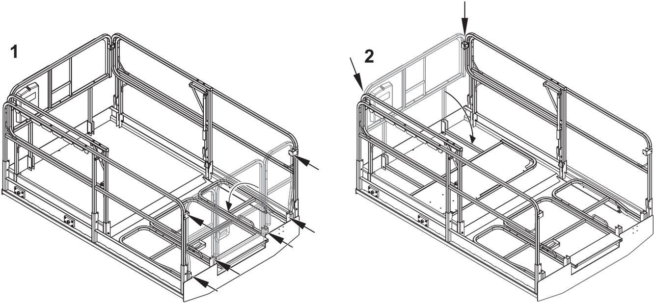
Figure 4-3. Platform Rails - Fold Down Sequence - Front/Rear Rails
