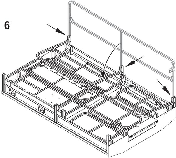
**Figure 4-5. Platform Rails - Fold Down Sequence - Main Platform Side Rails**
