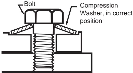
**Fig. 5** - Proper installation of compression washer and bolts.
