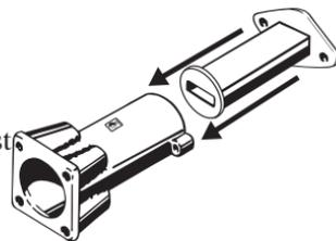
4. Place the driver on the post to be driven. Position the driver (**Fig. 4**) aligned centered to the post. If not aligned properly, damage could be caused to the driver or the post. Slowly squeeze the air throttle valve lever to start the driver. Opening the throttle valve slowly will prevent a violent start of the driver. Never tape, wire, etc., the throttle valve lever open.
