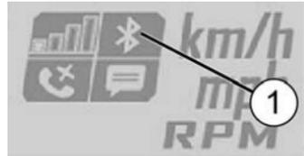
After successfully pairing the phone, the vehicle's digital gauge will automatically reconnect with the phone each time it is powered on and within range. No further action is required by the user at this point.
