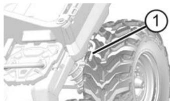
8. Firmly grasp a cargo box handle and slowly lift the front of the cargo box to dump the cargo.
