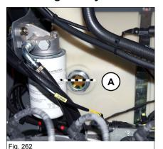
The oil level sight glass is located on the hydraulic oil reservoir on the left in the engine compartment.
