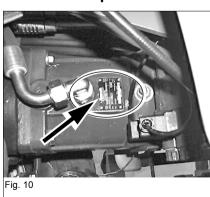
The type label (arrow) is located on the variable displacement motor (rear axle drive), on the right in travel direction.
