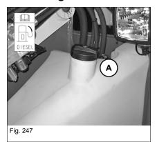
Filler inlet **A** of the fuel tank is located on the left side of the machine.
