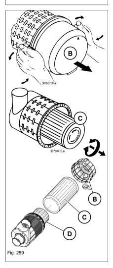
Indicator light  $\bf 69$  on the indicating instrument monitors the air-filter cartridge. Replace filter cartridge  $\bf D$  if this indicator light illuminates at the latest.
