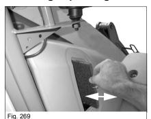
The dust filter is located behind the maintenance flap on the outside right of the cabin.
