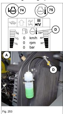
Temperature indicator  ${\bf D}$  (with acoustic warning) in the digital display on the indicating instrument monitors the cooling system.
