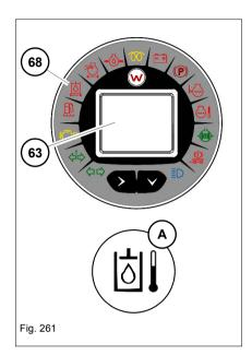
indicator light **68** on the indicating instrument monitors the return filter (dirt).
