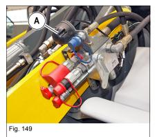
The machine is equipped with an optional 7-pole socket **A** (at the front left on the loader unit) for electrical attachments.
