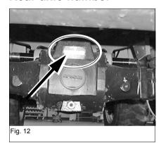
The type label (arrow) is located on the upper side of the differential housing, at the rear.
