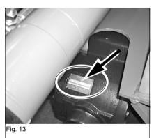
The type label (arrow) is located on the upper side of the differential housing, at the front.
