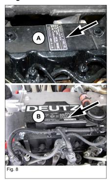
The type label (arrow) is located on the cylinder-head cover (engine).
