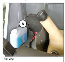
Reservoir A is located on the left in the engine compartment.
