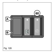
The push button for the rear wiper is located on the switch console on the right beside the steering wheel.
