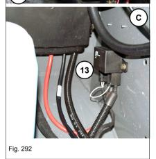
The relays (figure  $\bf A$  and  $\bf B$ ) are located under the switch console in the cabin, and in the engine compartment beside the main fuse box (figure  $\bf C$ ).
