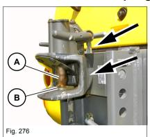
Cleaning and lubricating the trailer coupling
