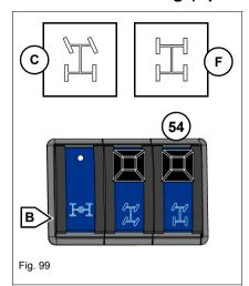
Front axle steering is used for fast transport and road travel.
