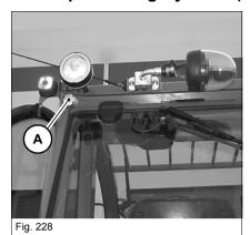
The backup warning system consists of signal transmitter **A** fitted at the rear top left of the cabin.
