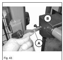
The door on the right can be opened to a gap and secured with the arrester to improve cabin ventilation!
