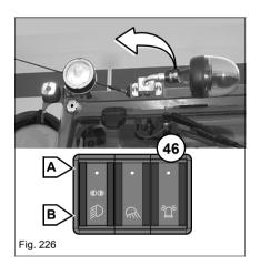
Switch **46** is located on the switch console on the left beside the steering wheel.
