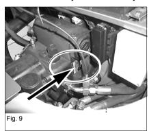
The type label (arrow) is located on the housing of the variable displacement pump (drive, next to where the pump is installed on the diesel engine).
