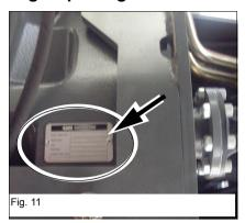
The type label (arrow) is located on the gearbox housing.
