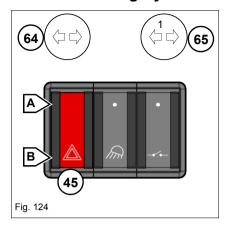
The hazard warning switch is located on the switch console on the left beside the steering wheel.
