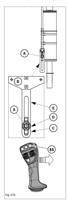
The bucket repositioning function can be used for performing cyclical work (for example for loading trucks) efficiently and with minimum impact to the material: by pressing a button, the attachment is automatically positioned from the tilt-out position to the preset work position (for example a horizontal bucket base).
