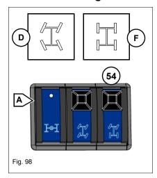
4 wheel steering is used for fast loading operations in confined spaces where only small turning circles are possible.
