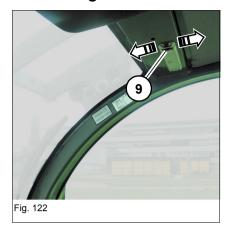
The interior light is located at the upper right on the cabin roof and is adjusted with switch **9**.
