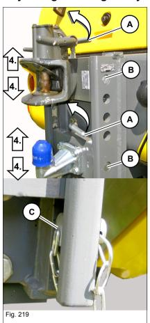
Before hitching a trailer, the height of the trailer coupling can be adjusted to the height of the trailer drawbar with the height-adjustable trailer coupling.
