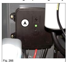
The main fuse box with the power relays and the preheating time control unit is located on the left in the engine compartment.
