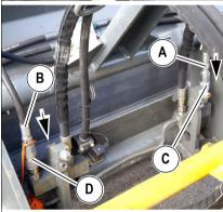
A hydraulic attachment (for example a multipurpose bucket) can be operated with the 3rd control circuit. Flexible lines **A** + **B** of the quickhitch quick couplers are connected to the attachment for this.
