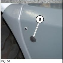
The hydraulic oil preheating is used as a cold-starting aid at temperatures below −5 °C (23 °F).
