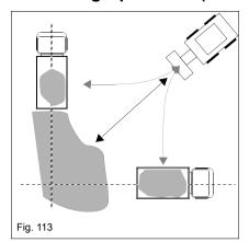
Reversing operation (change of travel directon without stopping) is only allowed in a secured job site for fast loading at low travel speed and lift heights.
