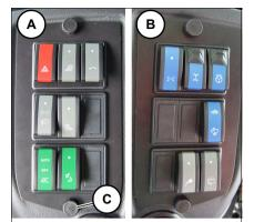
The relays and fuses are located under the switch console on the left  ${\bf A}$  and right  ${\bf B}$  in the cabin.
