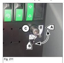
This option is used for securing the tilt ram if it is not supposed to be operated (for example when setting down material on high piles).
