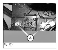
Reset the variable displacement pump to drive operation once towing the machine is over!
