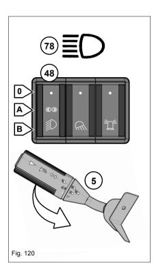
High beam and the headlight flasher are operated with multifunctional lever **5**. The multifunctional lever is located on the left of the steering wheel.
