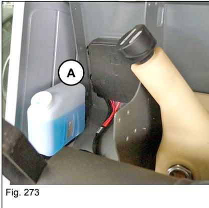
Reservoir **A** is located on the left in the engine compartment.
