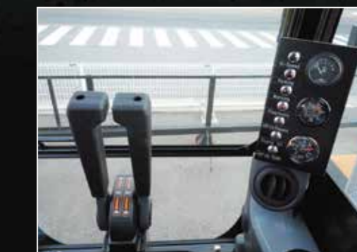
Two driving levers for MST-800VD, 1500VD, 2200VD and 3000VD
