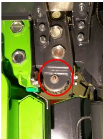
Figure 16 Telescoping chain pulley grease nipple
