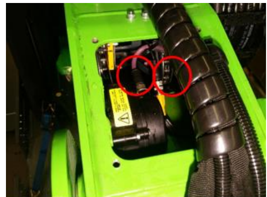
Figure 17: Leaf chain pulley greasing points in the front end of the upper boom.
