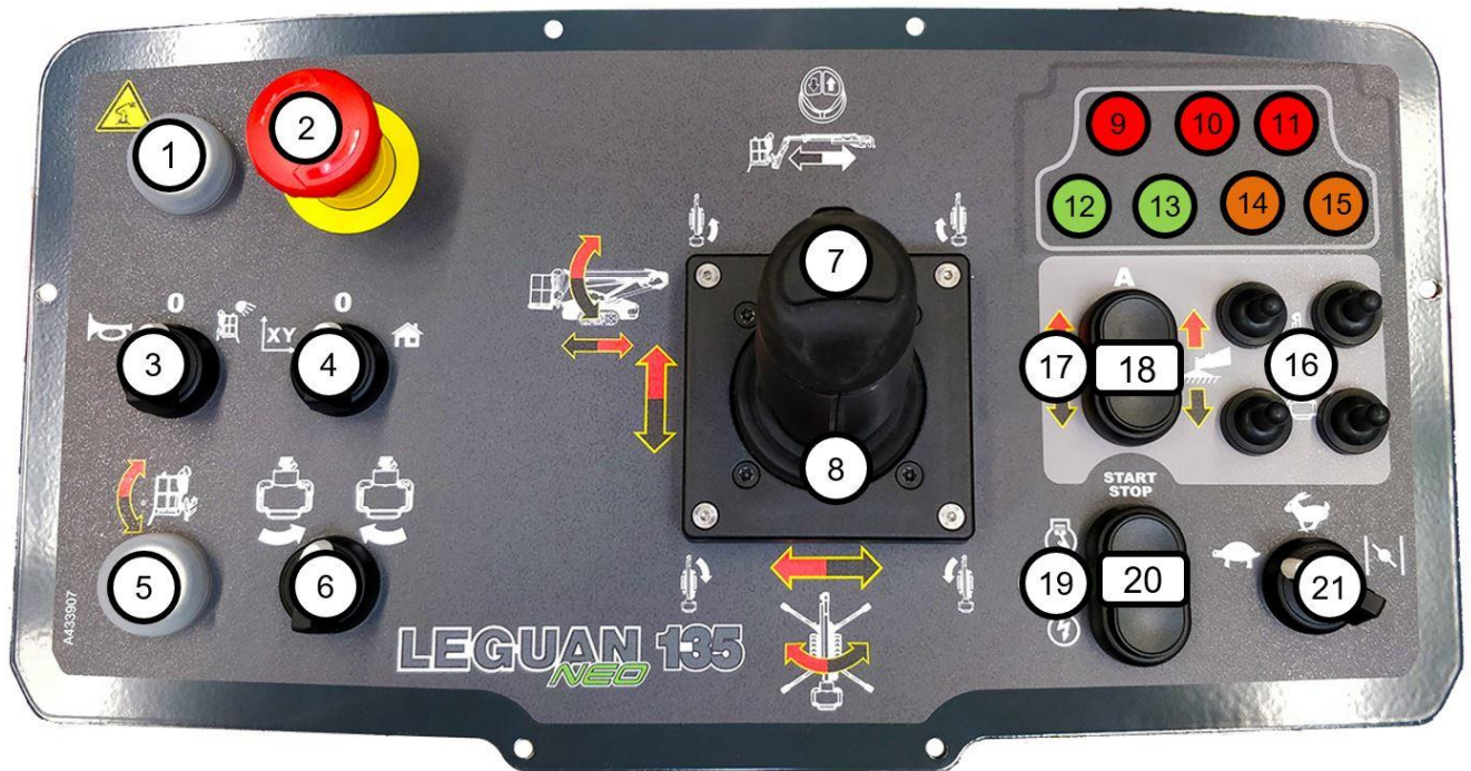
Figure 7 Platform control panel
