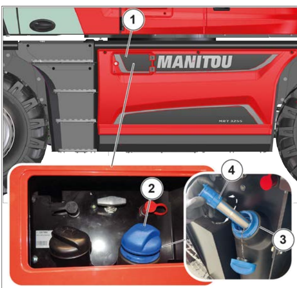
Figure 226: Checking and cleaning the DEF tank filler filter
