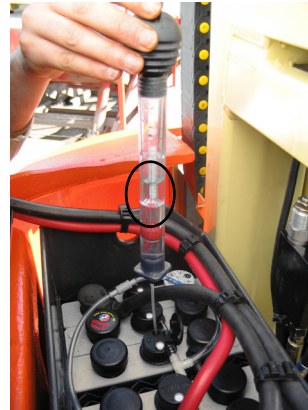
Figure 6-8. Measuring Electrolyte Specific Gravity
