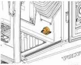
Battery disconnect switch in off position
