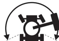
Note: When the drive enable system is in use, the machine may drive in the opposite direction that the drive and steer control handle is moved.
