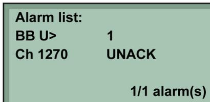
To see the other alarms, use the **UP** and **DOWN** push buttons to scroll in the display.
