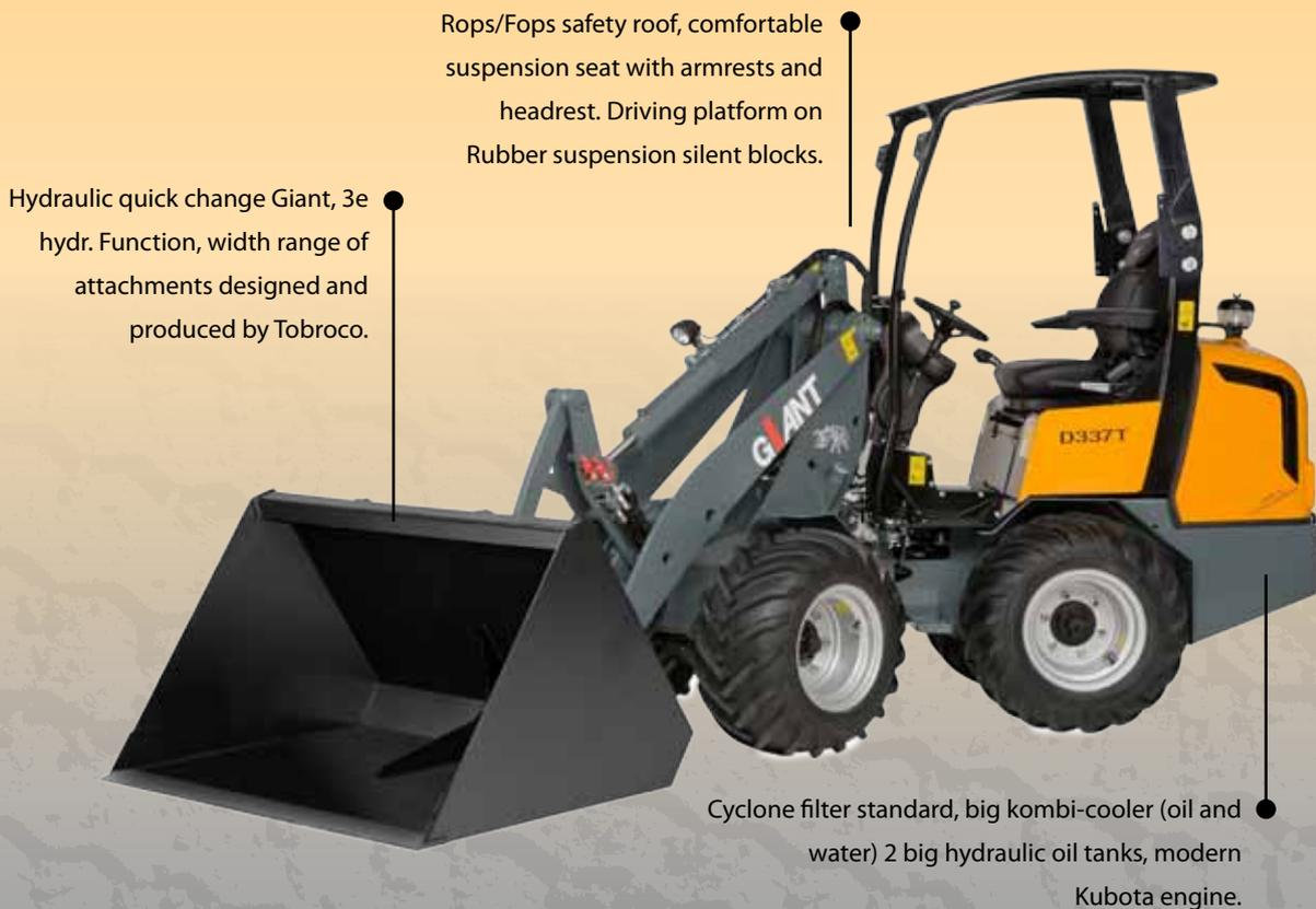
Rops/Fops safety roof, comfortable suspension seat with armrests and headrest. Driving platform on Rubber suspension silent blocks.
